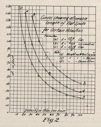
In working out the above relation between d and v no account has been taken of the action of gravity in bringing the mass down upon the rail with increased energy. The distance, equal to the distance of A below the center, approximately h/4, is so small that one might expect beforehand that the kinetic energy would be increased but little. Adding the term to account for this kinetic energy of the fall, M (2gh) Mgd<sup>2</sup>
