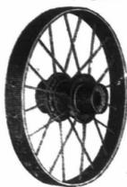
Made to fit your axle. Every farmer should have a set of these low, wide-tire, wrought-iron wheels for drawing hay, grain, corn, manure, stone, etc. They are lighter, stronger, and much cheaper than wooden wheels. Write for prices.
