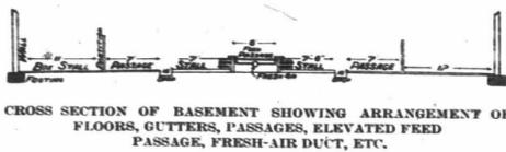
CROSS SECTION OF BASEMENT SHOWING ARRANGEMENT OF FLOORS, GUTTERS, PASSAGES, ELEVATED FEED PASSAGE, FRESH-AIR DUCT, ETC.
