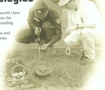
CCMAT tests and evaluates new mine action technologies. This prodder underwent testing in Cambodia.
