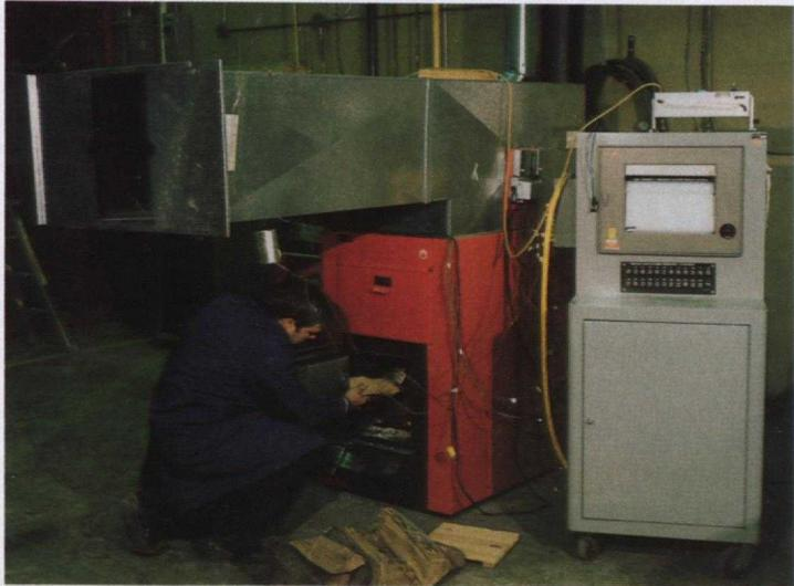
A wood-burning furnace with supplementary electric heating is being tested.
