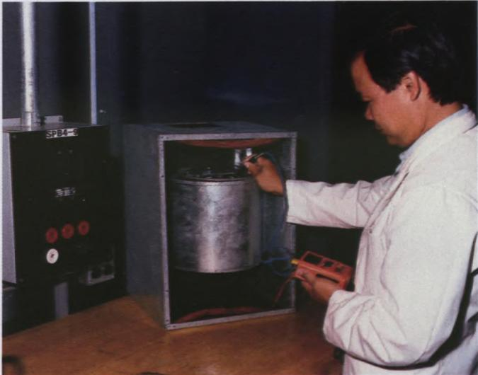
Recording the motor-casing temperature of a ventilator blower motor during operation.
