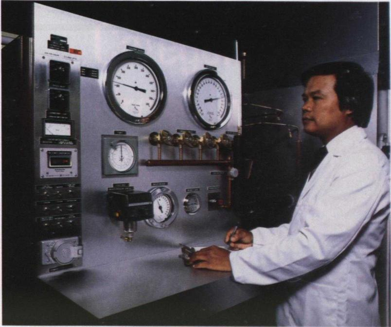
A refrigerant compressor undergoes a continuous maximum electrical current test.
