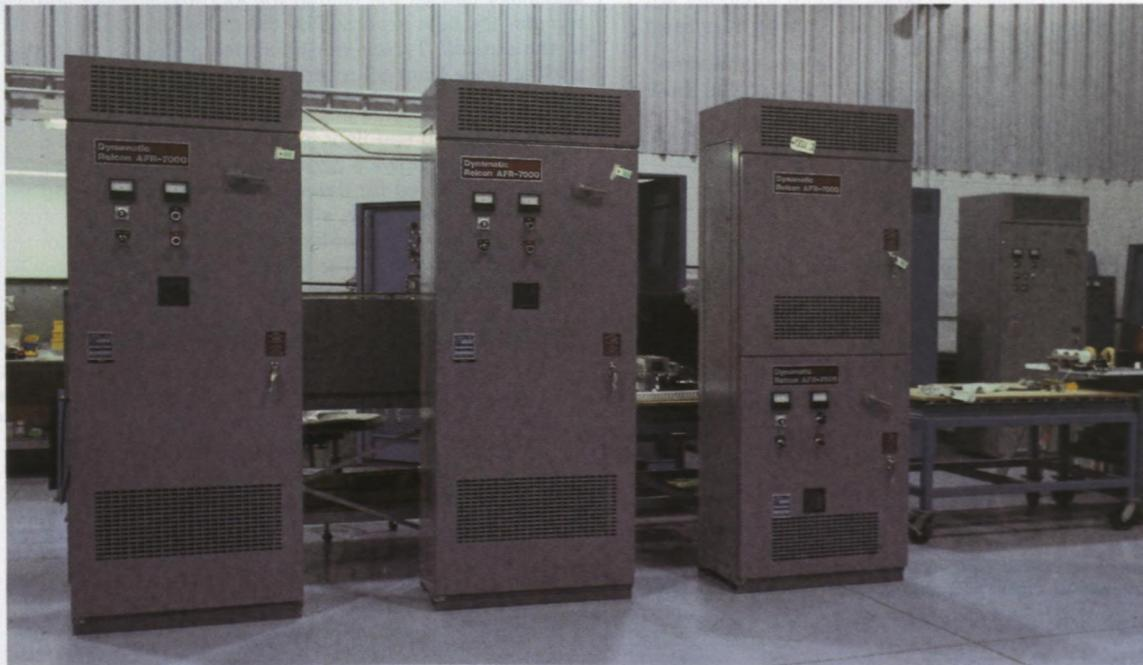
Variable torque adjustable-frequency Relcon drives are designed specifically for fan and pump applications.
