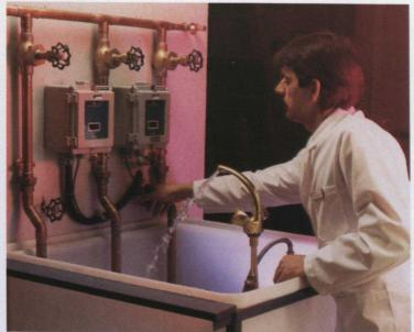
CSA technician measures the flow rate of a lavatory supply fitting.
