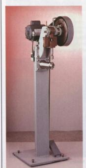
The TALOC fastening machine is ideal for fastening light-gauge sheet metal in the field.
