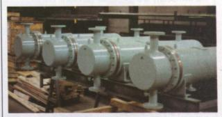
ISKO custom manufactures heat exchangers from such materials as carbon steel and copper for tough industrial applications.
