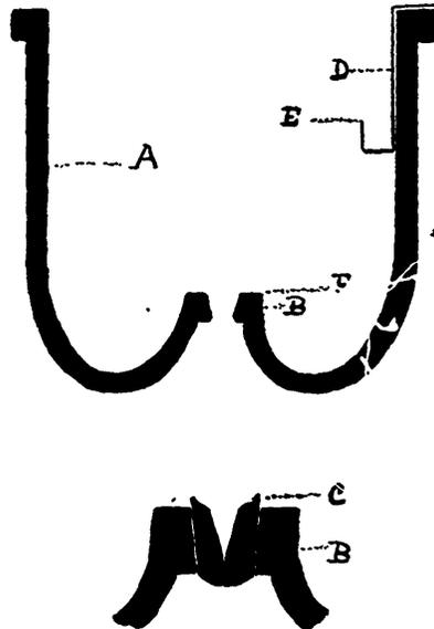
A is a cylindrical vessel of brass, 5 inches in each dimension; B is a re-entering cone,  $1\frac{1}{4}$  inches high, 1 inch diam. below and  $\frac{1}{2}$  inch at top. Into this are fitted (by ground-
