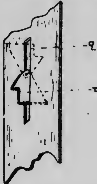
Fig. 17.—The catch in position.
