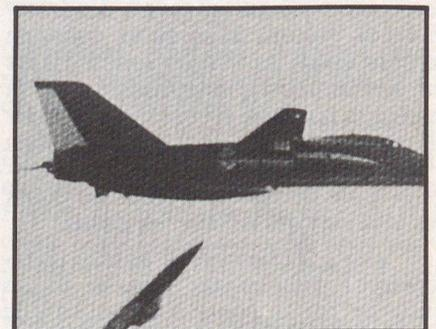
speed, the pilot increases his speed by a small amount and then excites a shake in the aircraft through what is known as a "stick pulse" — a rapid movement of one of the control surfaces (for example, the aileron). The amount of damping of the wing at the speed (that is, the degree to which the aircraft structure checks the vibration induced by the stick pulse) is determined from
