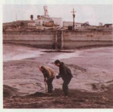
Reid Crowther Inc. Feasibility Study of methods to render the Con Mine tailings impoundment of toxic arsenic trioxide inert to the environment.
