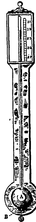
Ordinary upright barometer. A, Wood covering cup of mercury. B, Hole through which air acts.
