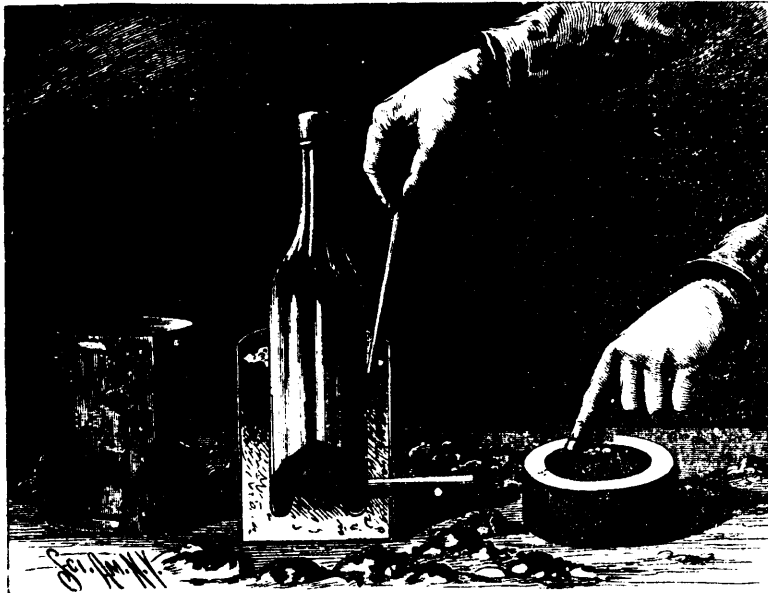
FIG. 11.—MAKING A BLOWPIPE FURNACE.
