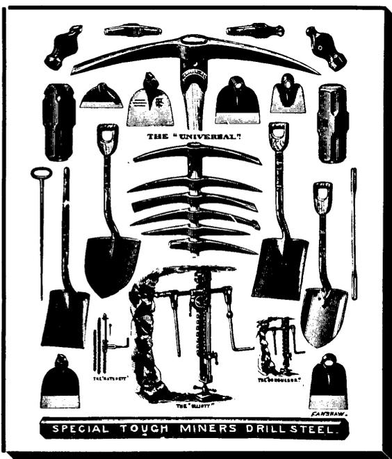
Picks, Shovels, Forks, Hoes, Axes, Hammers, Wedges, Files, Crow-bars, Etc. Hand and Power Boring Machines for all kinds of Rock and Coal. Special Tough Drill Steel.
