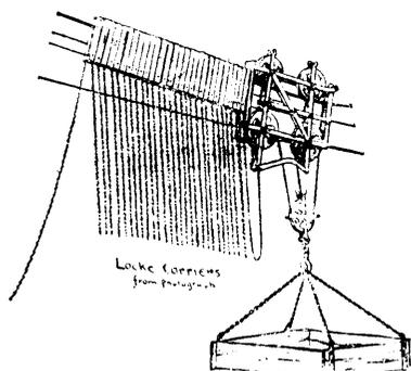
FIG. 3.—Chain Connected Fall Rope Carriers.
