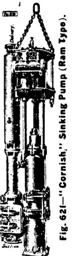
Fig. 621—"Cornish" Sinking Pump (Ram Type).
