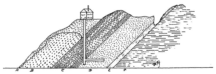
CROSS SECTION OF TENNY CAPE MINE-SCALE 100'=1 INCH.
