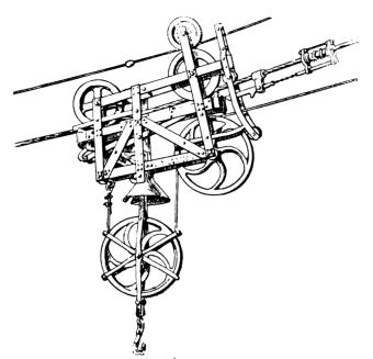
Fig. 2.—Harris-Miller Carriage and Fall Rope Carrier for Incline Cableways.
