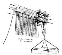
Fig. 3.—Chain Connected Fall Rope Carriers.
