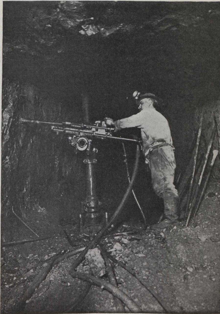
One-man (Leyner) drill, 5 9 th level, Conglomerate lode. Photo by O. Gardner. Calumet and Hecla Mine, Calumet, Mich.
