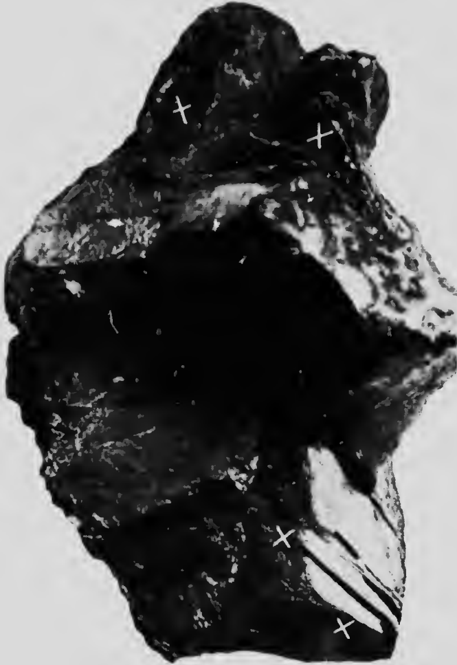
Canadian Graphite Ore: Pure Vein Graphite Exhibiting a Coarse Lamellar Structure.
