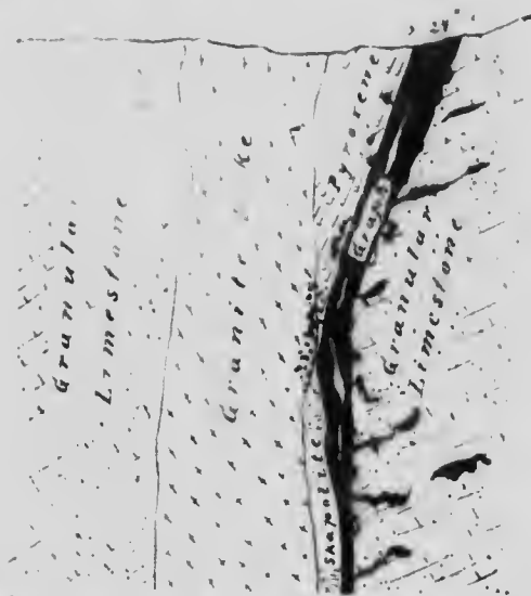
Fig. 9—Graphite Vein in Granular Limestone near Calumet Station, Can.
