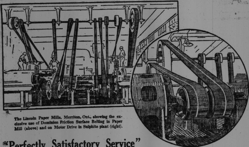
The Lincoln Paper Mills, Merriton, Ont., showing the exclusive use of Dominion Friction Surface Belting in Paper Mill (above) and on Motor Drive in Sulphite plant (right).
