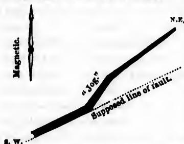
may have left the bed, and thus caused the appearance of the vein running in the former course of the bed along the line of fault, and also the greater regularity of the bed beyond the "Jog." This explanation is represented in Fig. 26."
