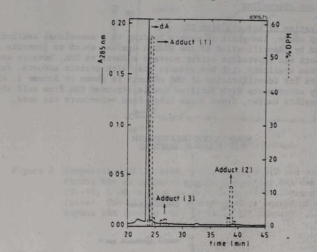
liquid chromatography (HPLC). The chromatogram (Figure 3) shows one major and two minor radioactive peaks, corresponding with different
