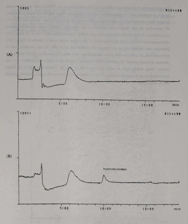
Figure 10 Determination of hydroxysoman in a waste water sample of a chemical factory. A : unspiked water
