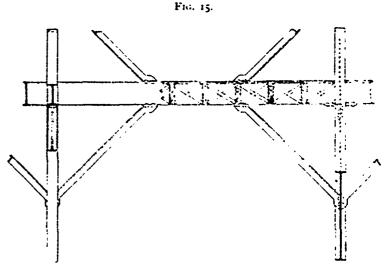
prevent vibration and preserve the stability of the structure. As a rule diagonals, preferably of T section, which divide the horizontal members into one-thirds (Fig. 15), will be found most advantageous; they are lighter than crossed diagonals or large angle gussets, quite as
