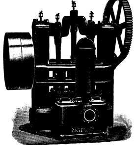
We illustrate in this advertisement a typical Pump for Mine Work. This is our Triplex Power Pump, fitted with tight and loose pulleys as shown in cut. It is the regular Triplex type with the three cranks 120 degrees apart; crankshaft and connecting rods are of steel; gears machine-cut from the solid; plungers of brass and all details carefully worked out. This Pump is especially adapted for service with Electricity as the motor power.
