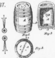
FIG. 1 Is an exterior view of Cask. FIG. 2 Is an interior perspective view of construction of the Cask. FIG. 3 Is a transverse horizontal section through middle of Cask.
