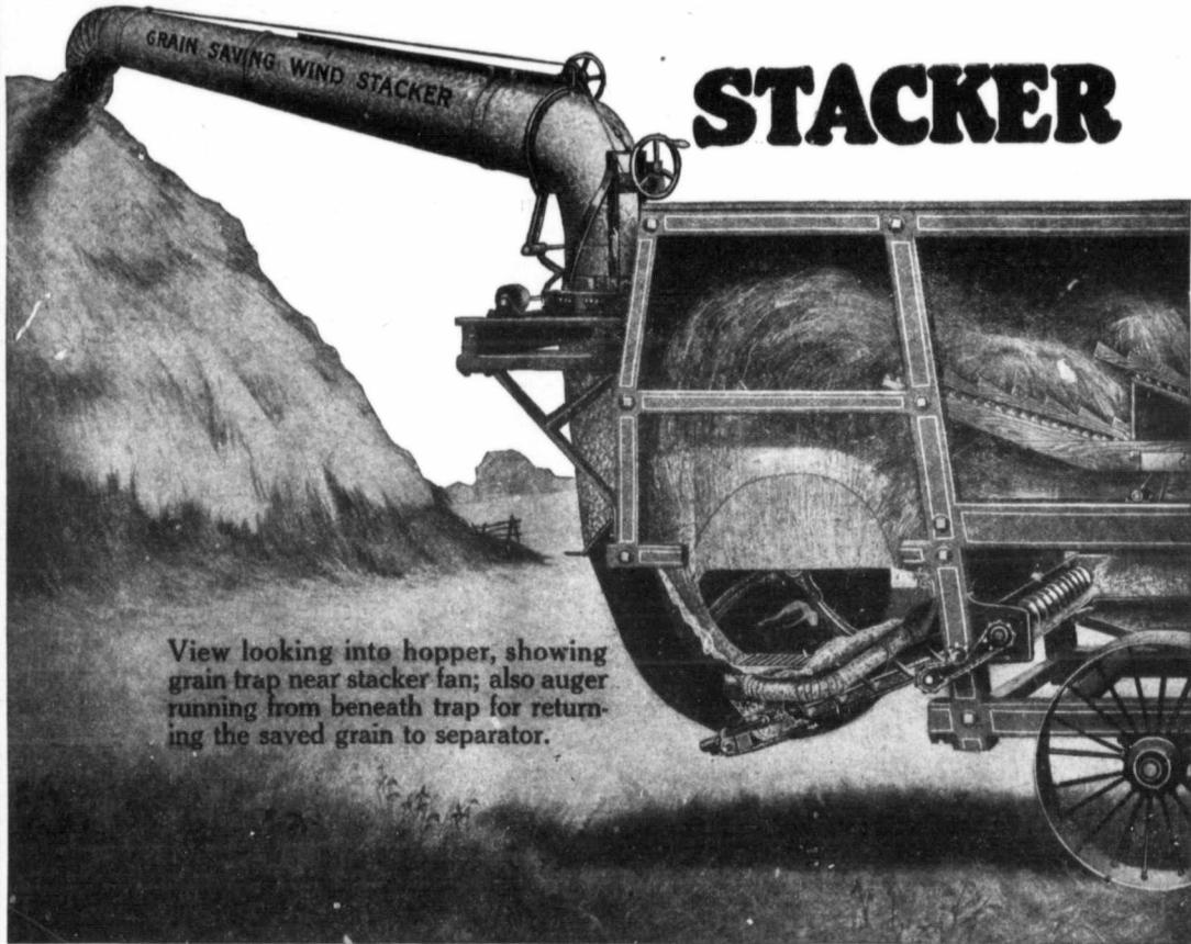
View looking into hopper, showing grain trap near stacker fan; also auger running from beneath trap for returning the saved grain to separator.
