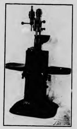
Bottling machine. The crown-cork machine.
