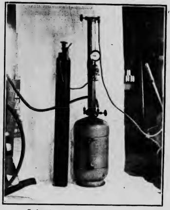
Carbonator. Gas drum and connections.
