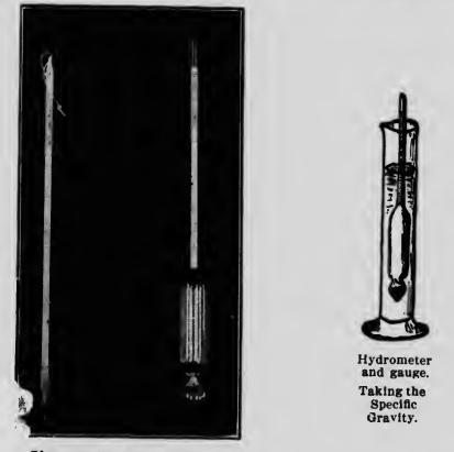
Thermometer and hydrometer.
