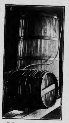
Filling a barrel from a tank.
