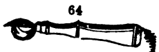
64 Sardine opener, to open tin boxes of sardines, preserved meats, preserves &c.
