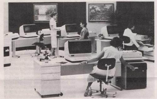
This version of the C20 consists of four local work stations (each with a screen and an electronic keyboard), five printers, each with a speed of 540 words/minute, a line-by-line printer with a speed approaching 8,000 words/minute and a central unit (or central module) containing the microprocessor.
