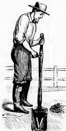
Showing the Digger with Blades closed upon the sand or dirt.
