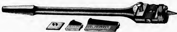
Showing the Bit with the Cutters off.
