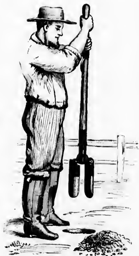
Showing the Digger with Blades open ready to be plunged into the ground.
