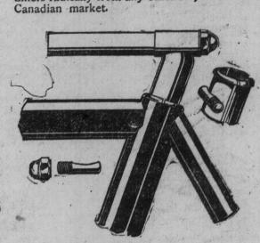
The working principle of this seat post fastener is shown in the accompanying illustration. The cotter key, milled away on one side to fit over expanding ring, is tightened so as to give the friction required to hold the seat post securely.
