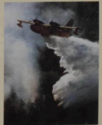
The chemical agent, Lorcon-Silvex, is mixed with the water that is picked up by the CL-215 twin-engined aircraft through a special on-board injection system developed by Aerospatiale of France and modified by Canadair Limited of Montreal, Quebec. When the mixture is released into the air, it becomes a foamy white blanket that clings together as it falls on its target.
