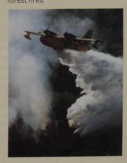
The chemical agent, Lorcon-Silvex, is mixed with the water that is picked up by the CL-2I5 twin-engined aircraft through a special on-board injection system developed by Aerospatiale of France and modified by Canadair Limited of Montreal, Quebec. When the mixture is released into the air, it becomes a foamy white blanket that clings together as it falls on its target.
