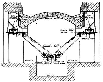
Fig. 1-Cross Section of Murphy Smokeless Furnace
