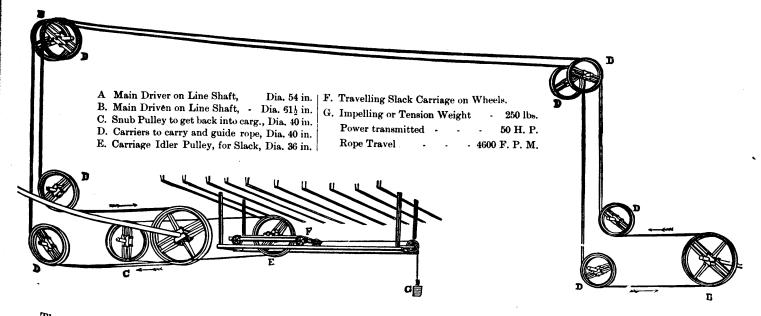
The above illustration shows the Dodge System of transmitting power by manilla rope and grooved hard wood of the same manufactured and erected by Dodge Wood Split Pulley Co., Toronto, and demonstrates fully the practicability of the system. That it may be clearly understood and appreciated, we give the following description:
