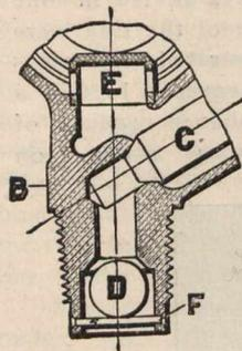
Fig. 2: Detail Sectional View of Shank; Showing Ball Check D, and Baffling Cap E.
