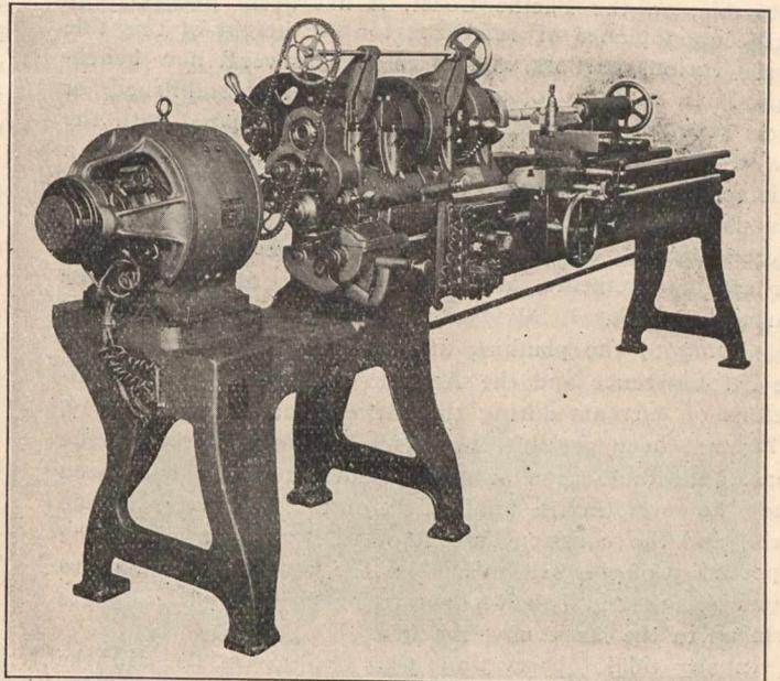
Fig. 3.—Lincoln Variable Speed Motor Applied to Lathe.
