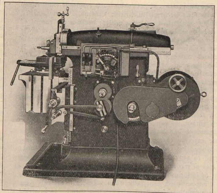
Fig. 4.—Two H.P. 5 to 1 Motor, Mounted on 16" Shaper.
