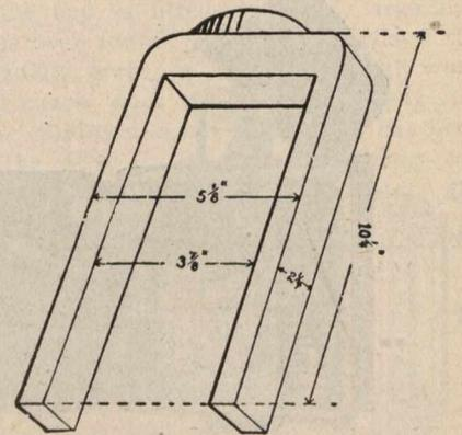
engines. For this purpose one of several styles of straps has been selected as an example. They are milling these straps all over and doing the work in remarkably good time.
