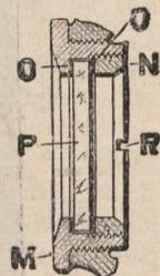
Fig. 3.—Detail Sectional View Showing Improved Construction of "Bull's Eye" sight-feed.
