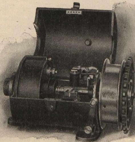
Fig. 1.—Stop Mechanism for Ordinary Steam; Reciprocating or Turbine Engine.
