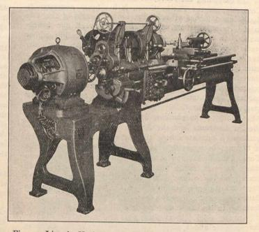
Fig. 3.-Lincoln Variable Speed Motor Appliel to Lathe.
