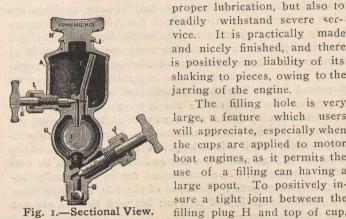
the plug is, provided with a lead washer I, which material, being softer than the brass upon which it bears, will readily conform to any irregularity that might exist between these bearing surfaces. It is almost impossible for this gasket to wear out, owing to the slight friction it is subjected to, but should the same wear, it can quickly and easily be renewed.
