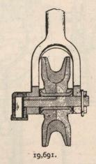
having grooved wear annulus, whose outer sides snugly fit and reliably hold the discs together, the whole combination, as shrown in the illustration, being such as to readily remove the portions subjected to wear.
