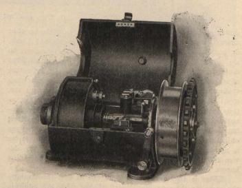
Fig. 1.—Stop Mechanism for Ordinary Steam; Reciprocating or Turbine Engine.
