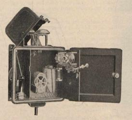
Fig. 2.-The Mine-A-Phone: Open View.
