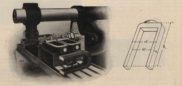
engines. For this purpose one of several styles of straps has been selected as an example. They are milling these straps all over and doing the work in remarkably good time.
