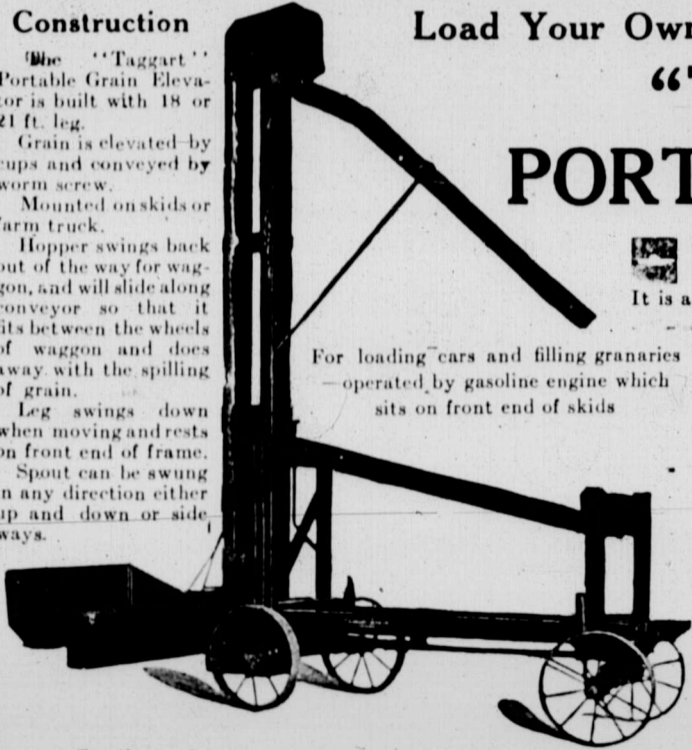
Cut shows elevator mounted on truck with leg up and hopper ready to receive grain.
