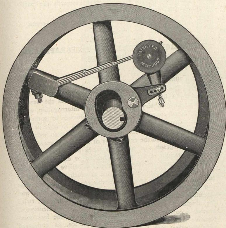
of its centrifugal force is carried by end pull on the flat leaf spring, so that the inertia of the weight is sufficient to prevent disturbance by the reciprocating motion of the valve gear, and the weight is so placed that it also gets the effect of inertia for quick regulation. The result is an extremely simple and powerful governor, in which there is not enough friction to prevent the governor from changing position almost instantly, and no possibility of racing when properly adjusted.
