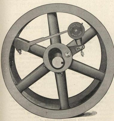
of its centrifugal force is carried by end pull on the flat leaf spring, so that the inertia of the weight is sufficient to prevent disturbance by the reciprocating motion of the valve gear, and the weight is so placed that it also gets the effect of inertia for quick regulation. The result is an extremely simple and powerful governor, in which there is not enough friction to prevent the governor from changing position almost instantly, and no possibility of racing when properly adjusted.
