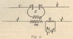
The receiver is constructed quite similarly to the transmitter, except that in a sense the connections are reversed, since in this case it is the open circuit in which the oscillations are set up and which forces its oscillations on the closed circuit of the secondary.
