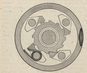
for needed repairs. The movement of the tool is a new one. Even a vertical motion of the handle will drive the drill, and two inches of motion is sufficient. In No. 6 size, there are twelve large teeth in the ratchet and five pawls which engage one at a time. Thus the pawls catch sixty times in a revolution, giving greater speed than other ratchets. The ratchet has been adopted by the United States navy, and is made in two sizes, No. 4 and No. 6, by the Armstrong Bros'. Tool Co., Chicago, U.S.
