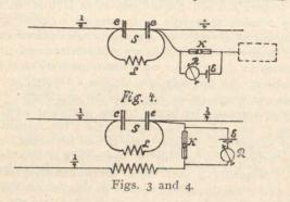
coherer disturbs the resonance; therefore, the second wire  $A = \frac{1}{4}$  wave-length is employed by which the resonance is restored and the working of the coherer is assured.
