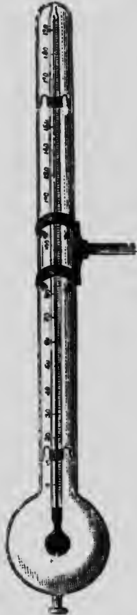
FIG. 49. — SOLAR RADIATION THERMOMETER.
