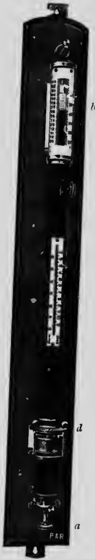
FIG. 41.—FORTIN'S STANDARD BAROMETER.
