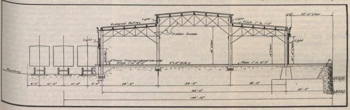
Cross Section of Timber Freight Sheds, Halifax Ocean Terminals.
