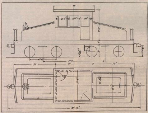
Electric Locomotive, Showing Dimensions, Montreal Tramways Company.
