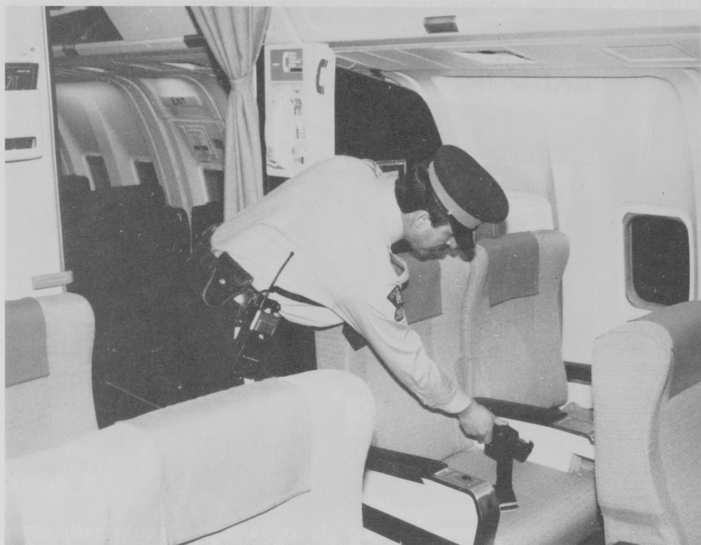
Inside a commercial aircraft, an EVD-1 operator uses a hand sampler to gather vapours for analysis, to determine if there are explosives on board.
