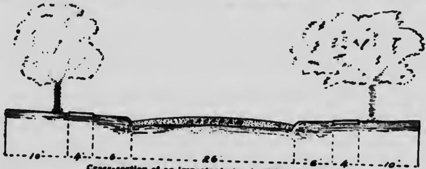
Cross-section of an important street without curbing.
