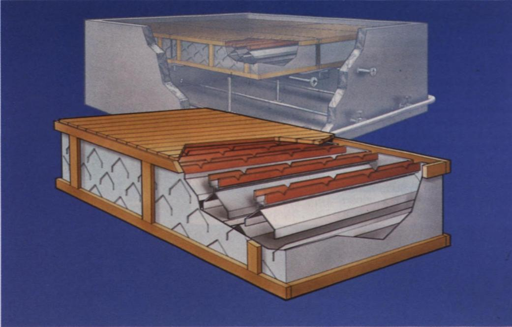
Illustration of a gas/water separator module in the foreground and the reactor container in the background.
