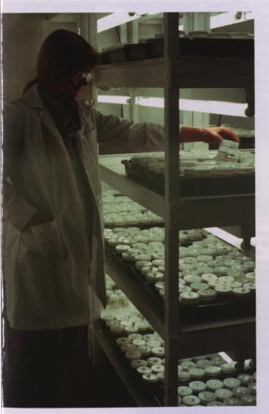
Growth chamber, culture of plant fragments. (Microelite Plant Laboratories Inc.)
