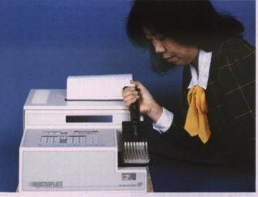
Technician working with the equipment used for the diagnosis of fungi that discolour and rot wood. (Forintek Canada Corporation)
