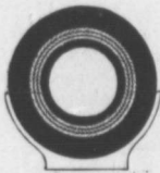
Section of Single Tube Carriage Tire, showing continuous thick walls and half of tire confined within the rim.
