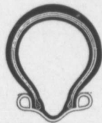
Section of 1 3/4-inch Dunlop Detachable Tire and Dunlop Tubular Metal Rim for Carriages, showing the thin flexible sides and thickened tread, and small portions of tire confined within the rim.
