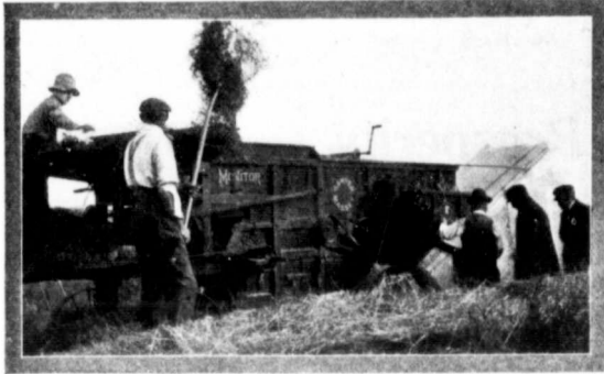
Sawyer-Massey Monitor Clover Huller at work on Mr. Irvine's Farm, Neopawa, Man. threshing Alfalfa. Mr. Irvine pitching. Shows very plainly the Recleaning attachment on the left side.
