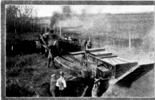
Sawyer-Massey Monitor Clover Huller at work on Mr. Irvine's farm, Neepawa, threshing Alfalfa, showing the complete rig at work, and also showing the Recleaning attachment.
