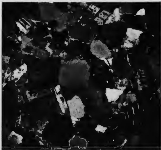
B. PHOTOMICROGRAPH OF THIN SECTION, (X 30 D.I.A.M. - N. CO. S. CROSSED) GRANITE, WESTERLY, RHODE ISLAND.
