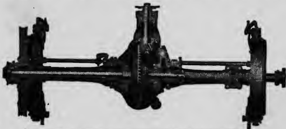
Section of rear axle showing spiral bevel driving gears, brakes and wheel bearings.
