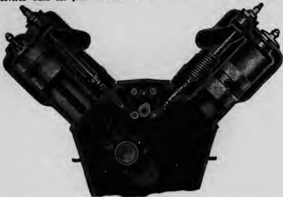
Section of 8-cylinder V-type motor showing valve rocker arm mechanism, water jackets and gas passages.
