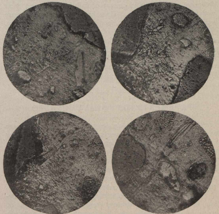
Fig. 1.—Examples of Shear Planes in Under-water Concrete (x110).
