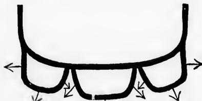
In above Flue Construction there are **NINE** Surfaces Radiating Heat, Increasing the Heating Capacity with the same amount of fuel.
