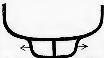
In above Flue Construction there are **Four** Surfaces Radiating Heat.
