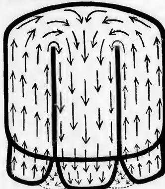
The above Bottom Flue Construction causes the Heat to go to the Outer Surfaces, Largely increasing the Heating Capacity and Economizing in Fuel.
