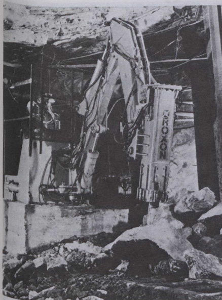
Perforateur hydraulique TM16, de Teledyne Canada Mining Products de Thornbury (Ontario).
