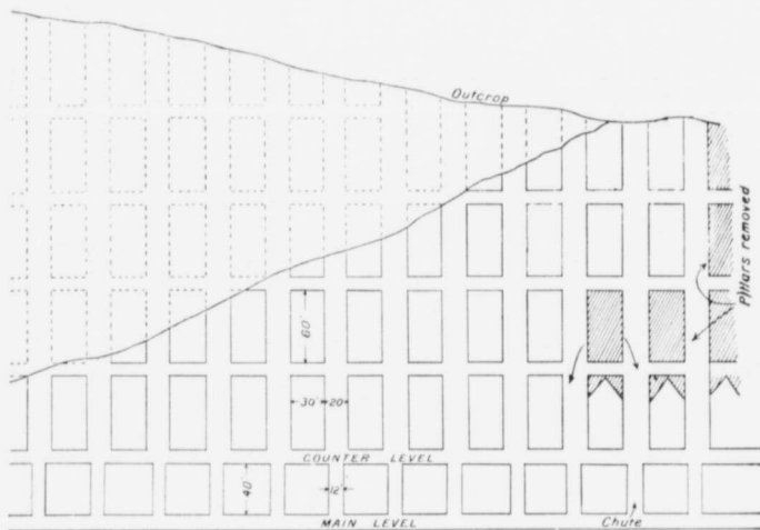
SKETCH SHOWING METHOD OF WORKING, DAVENPORT MINE
